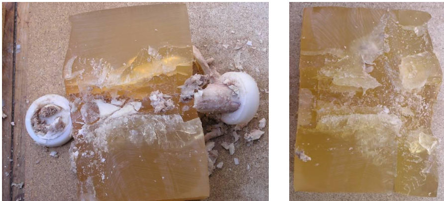
Fig. 6 Damaged gelatine model with bone fragments after impact of rifle projectile 7H6 of micro-calibre round 5.56x45
